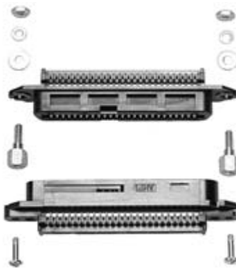
Screw Lock Hardware Kit Part Number 552568-1 (For rear panel mount applications, max. panel thickness shall be .062 [1.57].) (One kit required per assembly)
